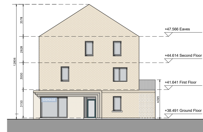
DUPLEX BLOCK F SIDE ELEVATION (WEST)
