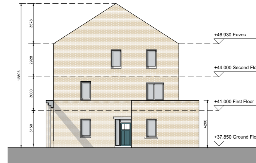
DUPLEX BLOCK G SIDE ELEVATION (WEST)
