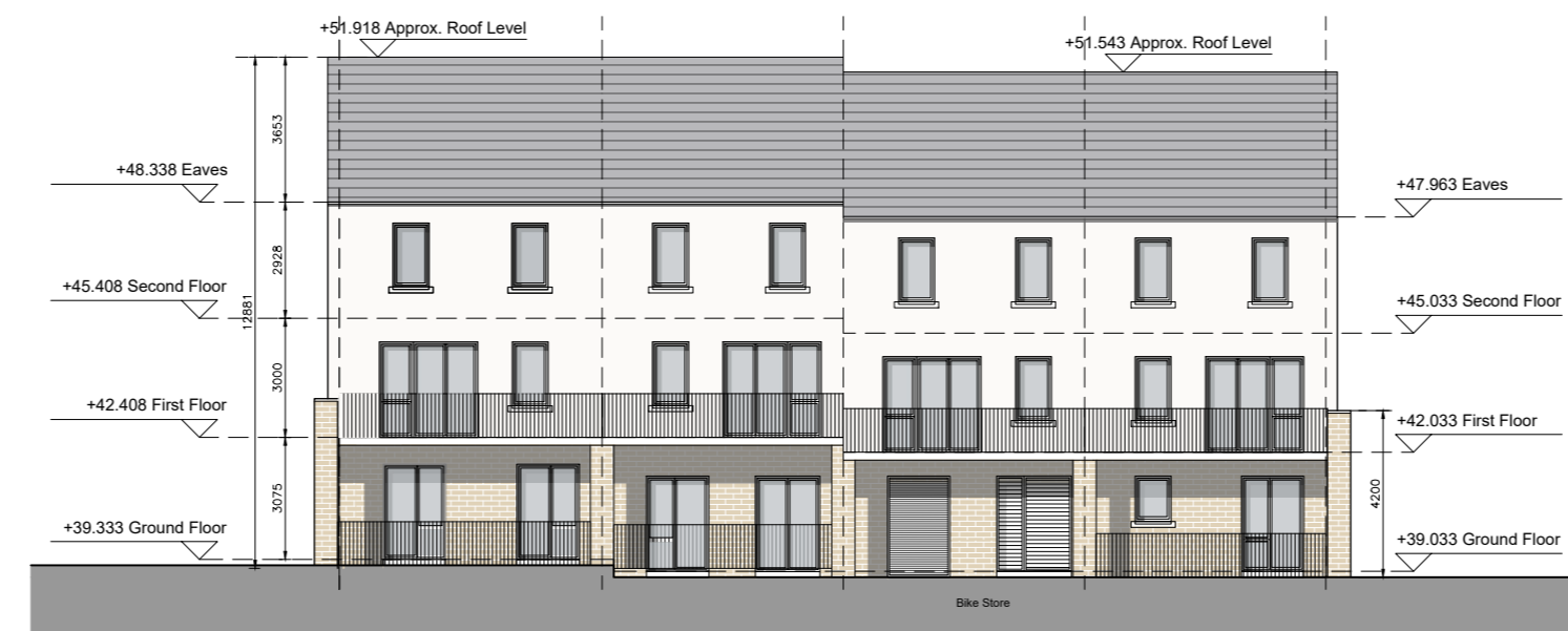
DUPLEX BLOCK I REAR ELEVATION
