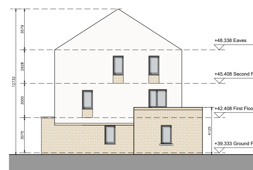
DUPLEX BLOCK I SIDE ELEVATION (NORTH)
