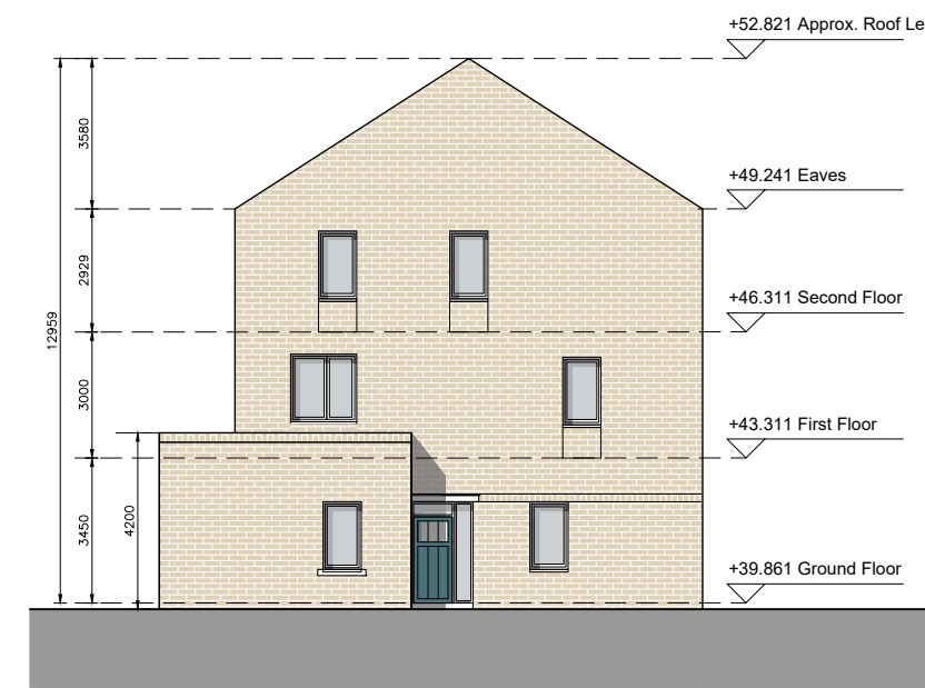
DUPLEX BLOCK R SIDE ELEVATION (WEST)
