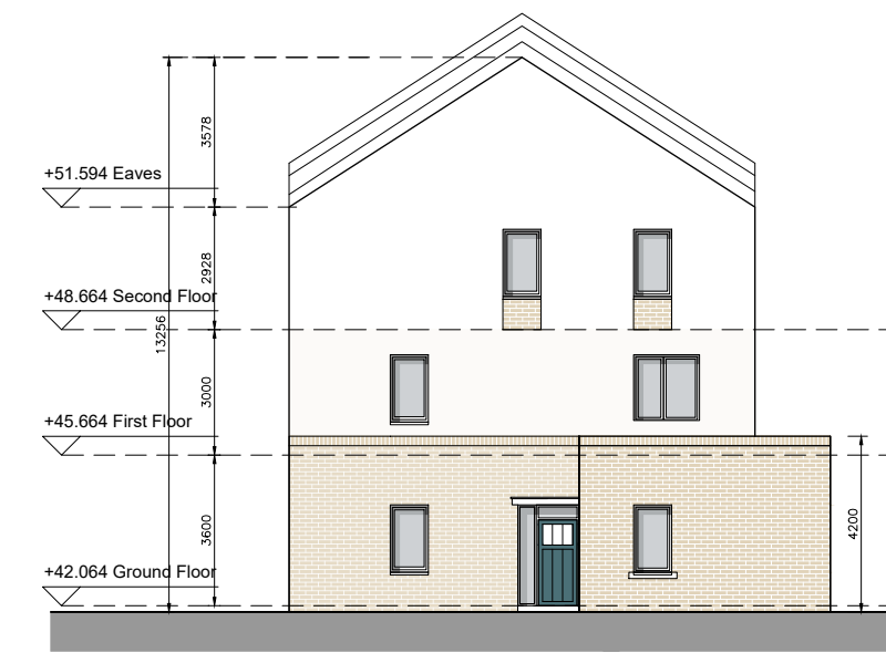
DUPLEX BLOCK C SIDE ELEVATION (NORTH)
