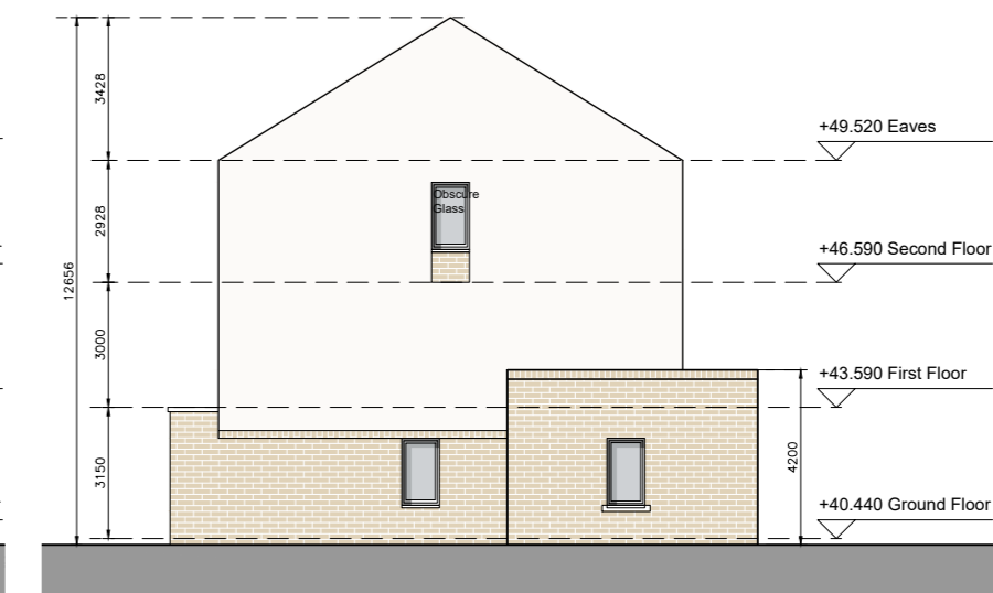
DUPLEX BLOCK J SIDE ELEVATION (NORTH)
