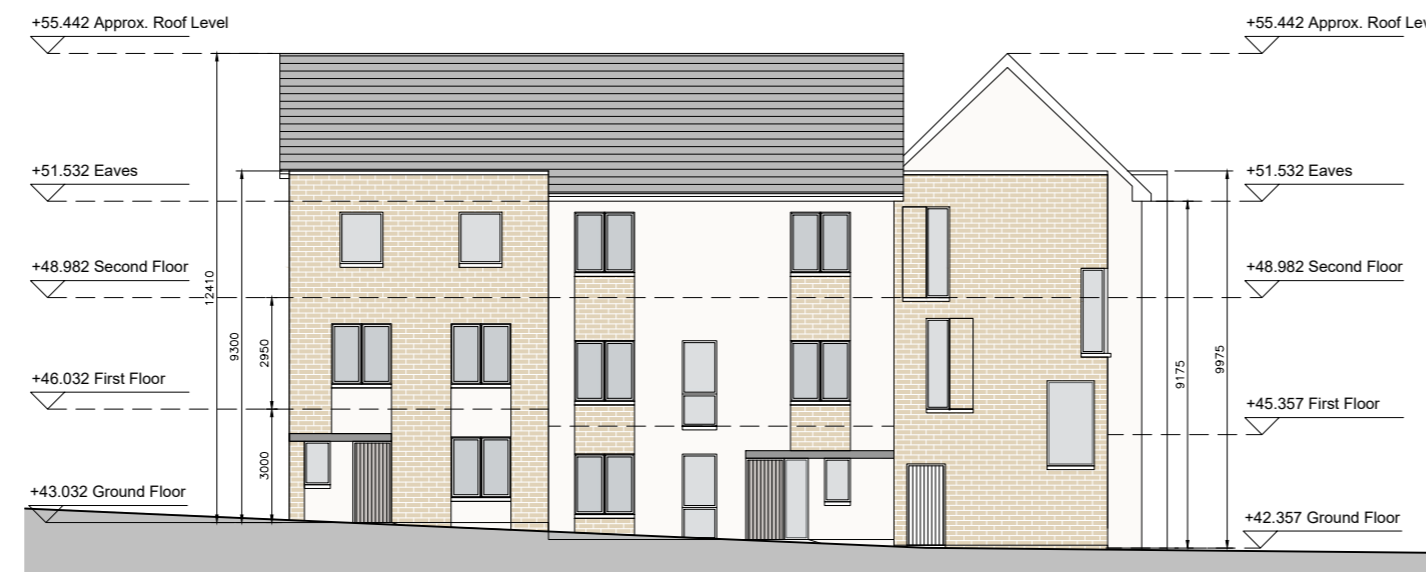
DUPLEX BLOCK U STREET ELEVATION (LONG)
