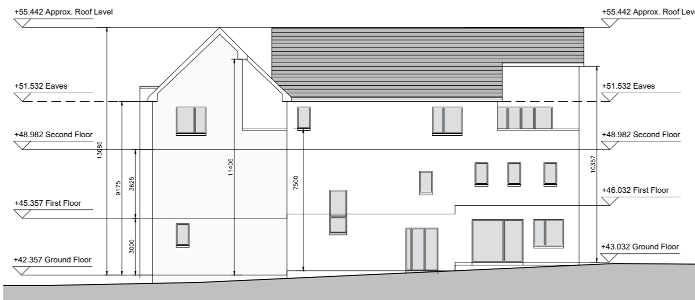
DUPLEX BLOCK U REAR ELEVATION (LONG)
