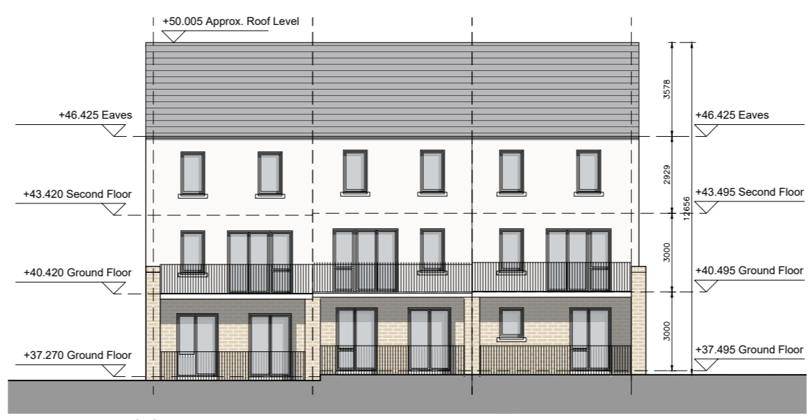
DUPLEX BLOCK H REAR ELEVATION
