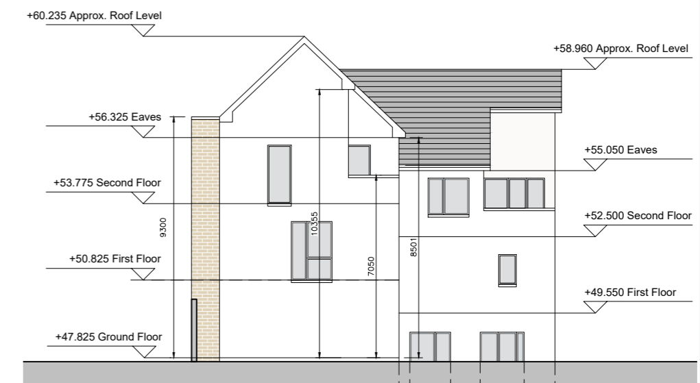
DUPLEX BLOCK S REAR ELEVATION (SHORT)
