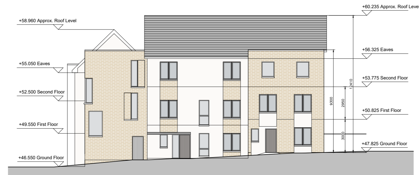
DUPLEX BLOCK S STREET ELEVATION (LONG)
