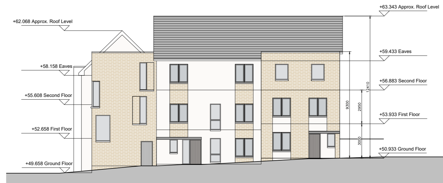
DUPLEX BLOCK T STREET ELEVATION (LONG)
