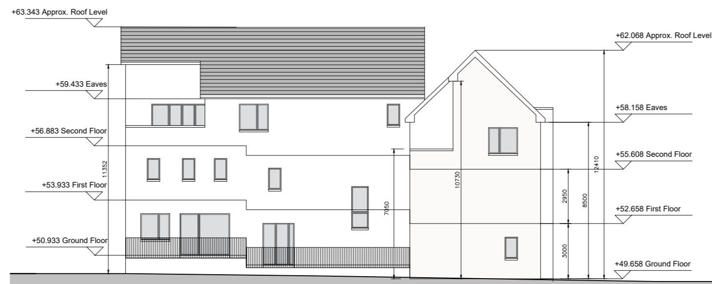
DUPLEX BLOCK T REAR ELEVATION (LONG)
